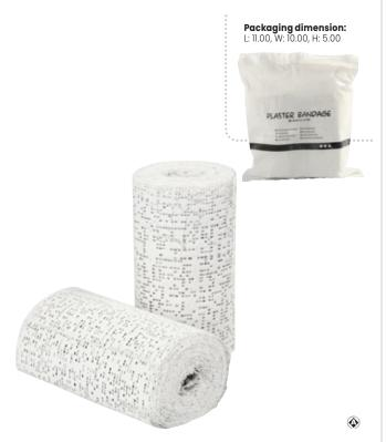
**Plaster Bandage** A gauze bandage impregnated with plaster - dip in water for few seconds to make it flexible (pasty) and workable. The plaster bandage can be cut into small pieces or used directly from the roll - can be used on plastic, glass, papier-māché, netting etc. If applied directly on skin - apply a thin coat of Vaseline before application, L: 2,7 m, W: 10 cm.
